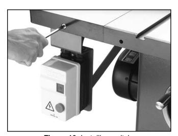
Figure 10. Installing switch.
